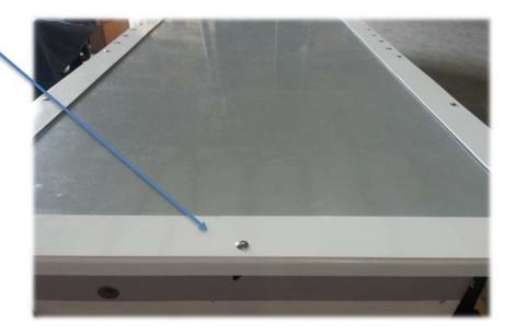
Step 8: Replace the 18 black knobs around bed and tighten securely.
