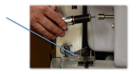
Step 6: Locate flat side of drive motor shaft, align with mark on coupling.
