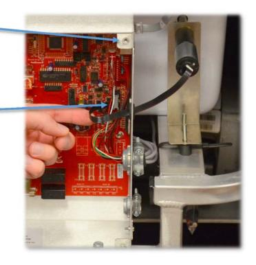
Step 4: Remove two drive shaft lock screws that hold the drive motor to the drive shaft.
