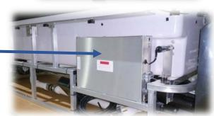
Step 9: Install the right side and foot panels with the 6 thumb screws.
