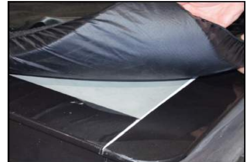
Step 6: Unsnap and remove cover sheet and comfort pad
