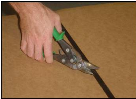
Step 1: Using Tip-Snip snip packing bands
