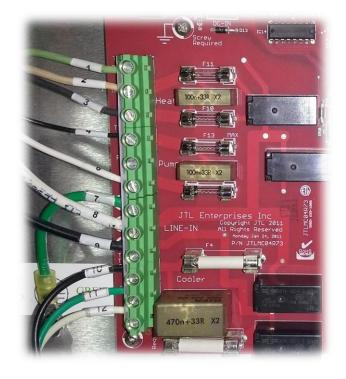
Step 9: Plug in the 4 plugs along the right side of the circuit board.
