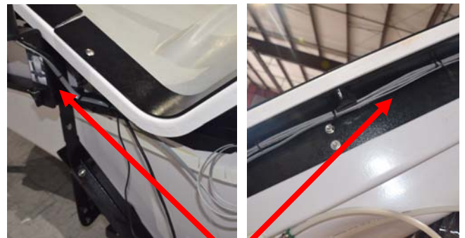
Secure wires and communication cable as shown with supplied tie wraps
