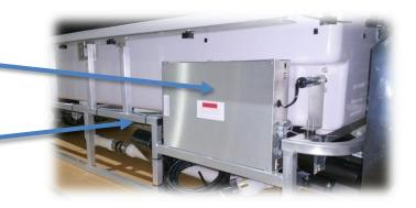
Step 12: Install the right side panel with the 4 thumb screws.
