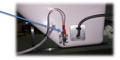
Step 10: Carefully insert plug through wire clamp into control box and re-plug the red connector onto circuit board. Then tighten wire clamp on control box
