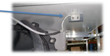
Step 7: Cut all 9 tie wraps holding harness to frame with wire cutters, then remove complete harness from bed
