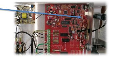
Step 11: Using the 9 supplied tie wraps, attach the wire harness to frame in the same orientation as the original
