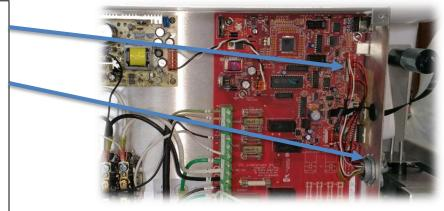
Step 5: Remove the two liquid level sensor wire connectors from sensor at the sump of tub
