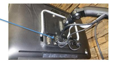
**Step 12**: Attach cable cover to the back of the touch screen with two screws.
