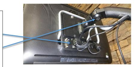
**Step 5**: While holding the touch screen, remove bottom cap. Lift touch screen up and carefully set on the bed.
