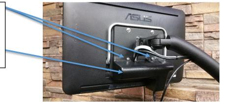
**Step 4**: Disconnect all wires from the back of the touch screen.
