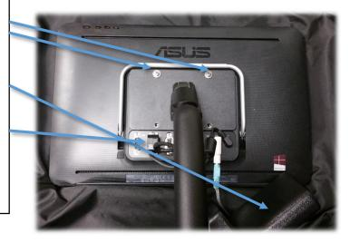
Step 4: Remove touch screen arm from bed frame. Place old and new touch screens face down on the bed.
